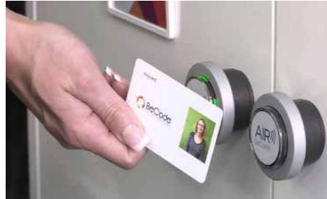
The lock is very easy to operate as it simply rotates to open and lock. Group access to a particular area or individual access can be easily managed and amended. Fixed users can have access to a designated locker, or temporary users in an agile environment can select and activate any free locker using their keycard or transponder device. Access to lockers can be removed immediately if a keycard
